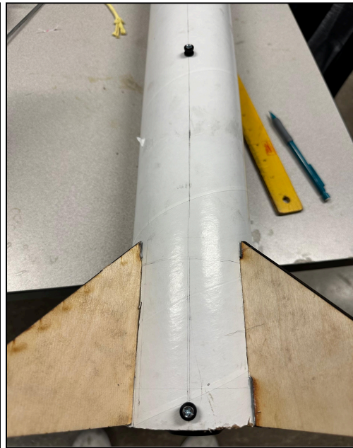
Figure 13: Drilling the rail buttonholes Figure 14: The completed rail buttons on the rocket on the same line of axis
