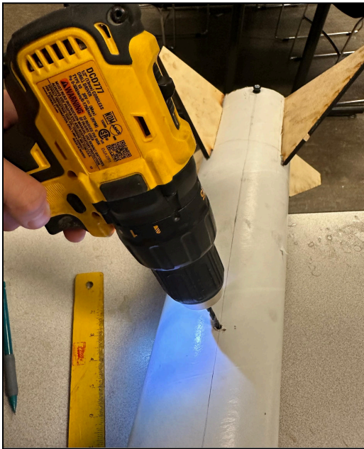
Figure 13: Drilling the rail buttonholes Figure 14: The completed rail buttons on the rocket on the same line of axis
