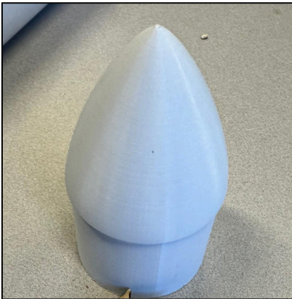
Figure 6: The 3D printed Nose Cone after taking off the tree supports
